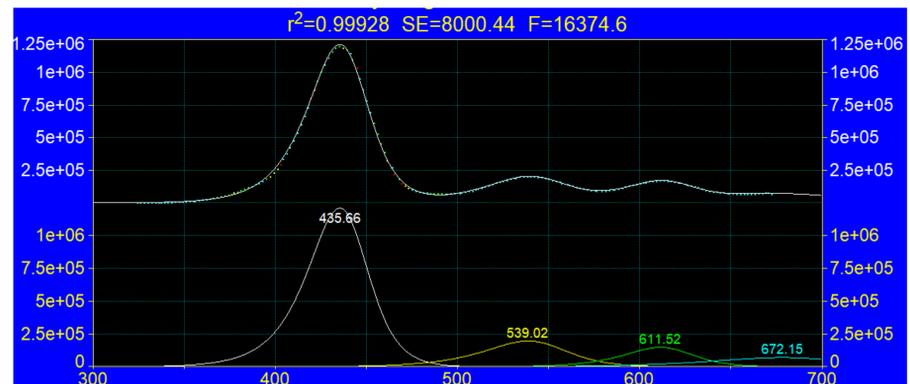
Fig. 3. Curve fitting results for the whole glow curve of alumina sample irradiated at 10 Gy dose.
