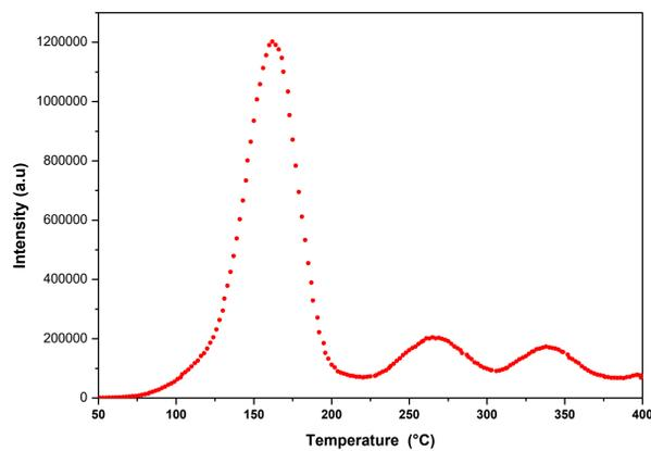
Fig. 1. Glow curve of sintered alumina pellets irradiated at a dose of 10 Gy.
