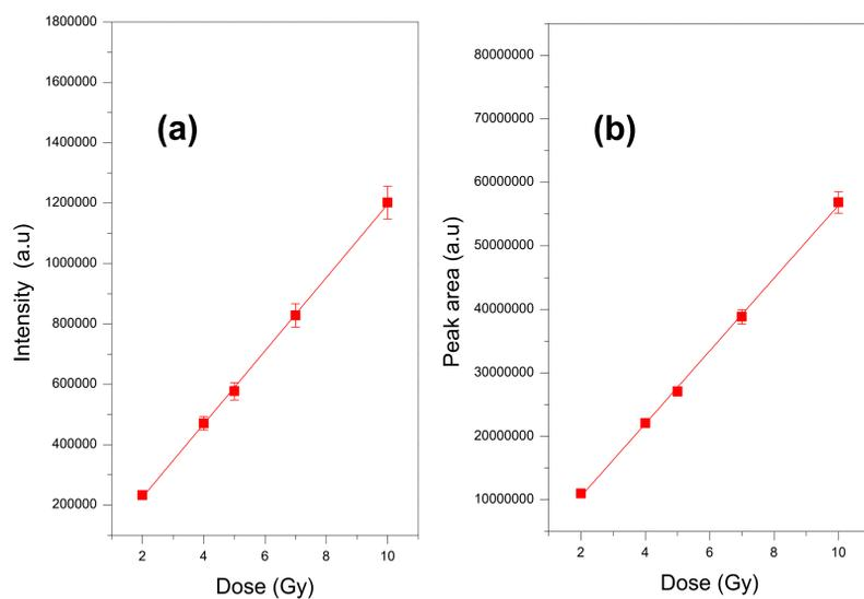
Fig. 4 Linear response of the material with doses from 2 to 10 Gy. The squares represent the experimental data while the line represents the linear fit.
