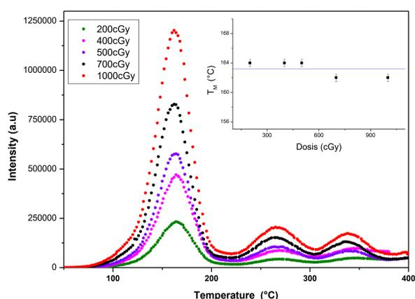
Fig. 2. Glow curves of alumina samples recorded at 5°C/s after irradiation at different doses. The inset shows the change in the position of the main peak with irradiation dose.
